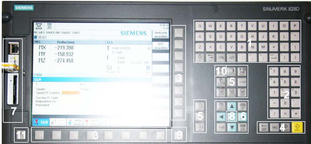
Img.5-2: Control panel
