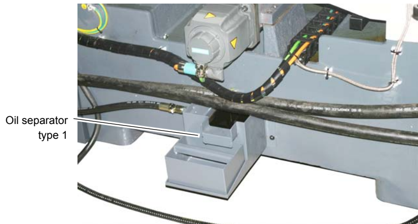
Img.3-16: Oil separator of the coolant / lubricant tank type 1
