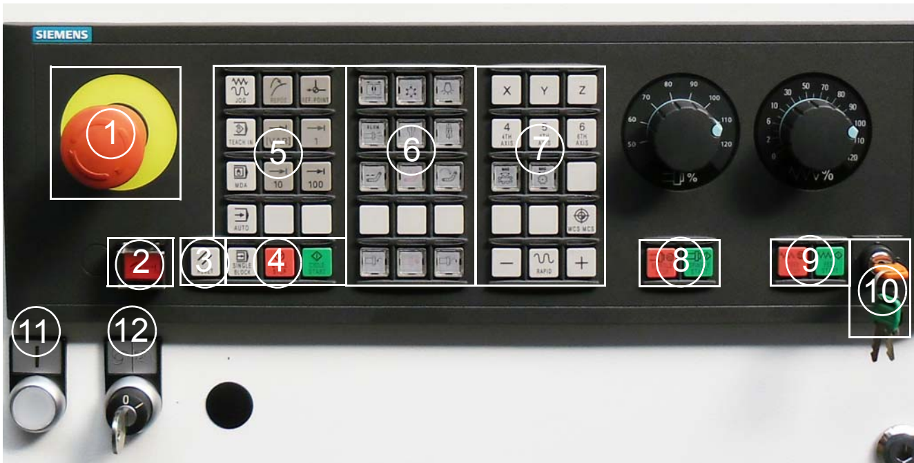
Img.5-3: Machine Control Panel
