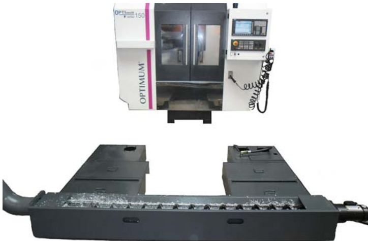
Img. 10-2: Cooling lubricant tank
