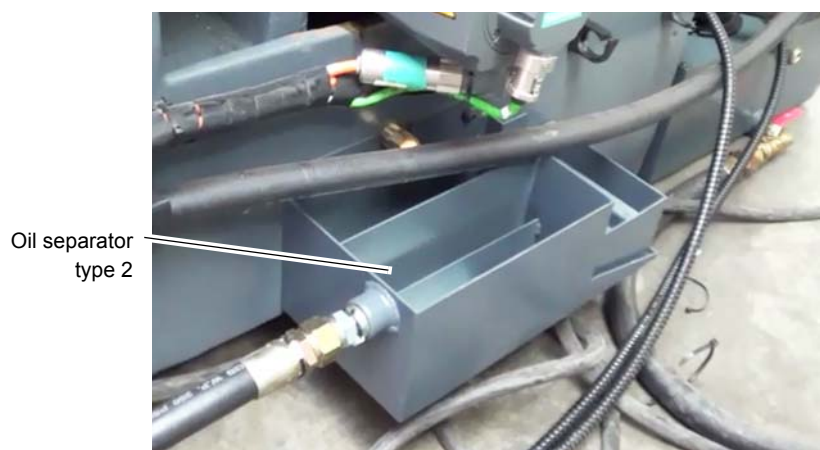
Img.3-17: Oil separator of the coolant / lubricant tank type 2
