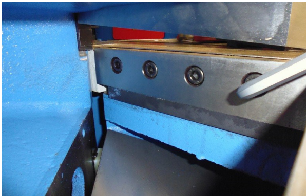
Fig. 21: Unscrewing of the screws of the lower knife
