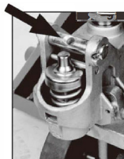
Fig. 6: pin mango Insertar
