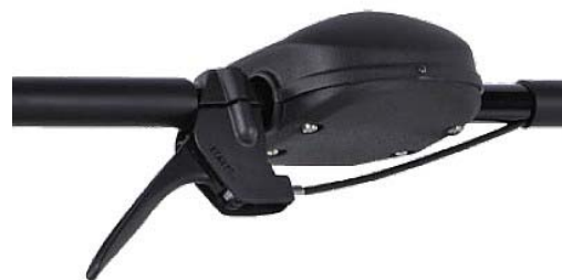
Fig. 8: Lever for lifting the suction lip
